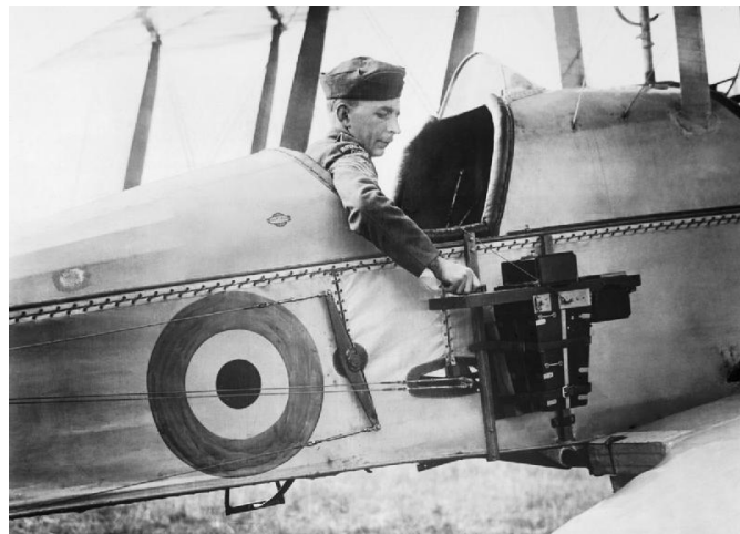
Figure 4: A B.E.2c reconnaissance aircraft of the RFC (Royal Flying Corps) with an aerial reconnaissance camera fixed to the side of the fuselage, 1916 (Wikimedia Commons).
